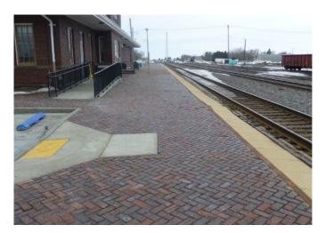
Figure 2-1. At-Top-of-Tie Platform Showing New Brick Pavers That Did Not Constitute an Alteration. Source: USDOT
