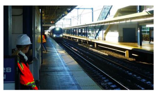
Figure 4-4. Double-Track Railroad Side Platform Configuration. Source: USDOT
